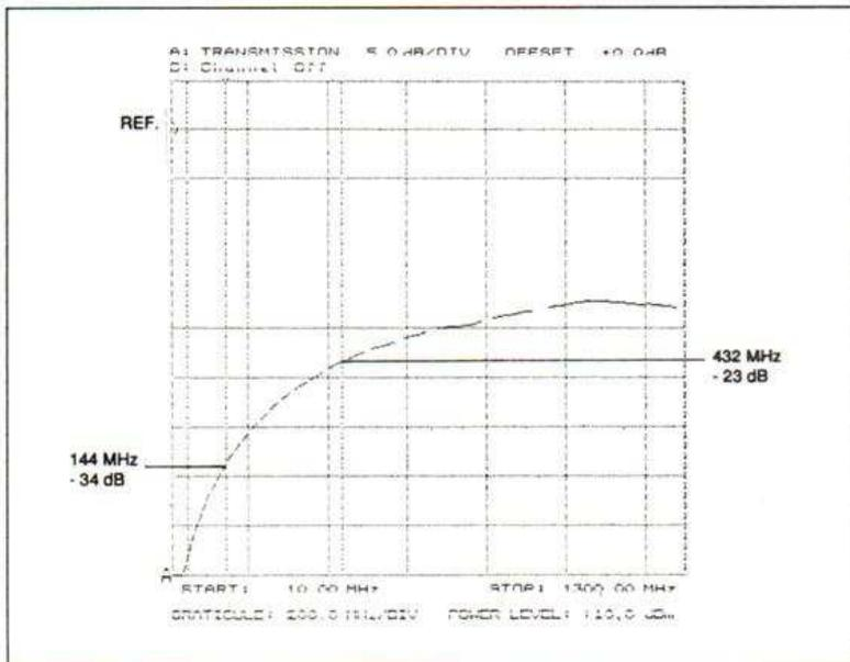
**Fig. 11. – Isolation E/R ; relais ISKRA TRK 3113.**
