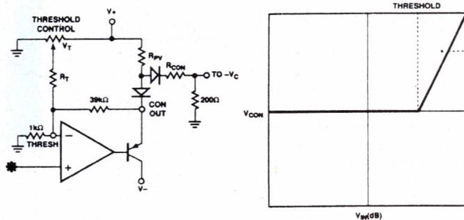
\*UPPER LIMIT CAN BE FIXED BY VALUE OF PULL UP RESISTOR ( $R_{PV}$ ) CONNECTED TO POSITIVE SUPPLY
