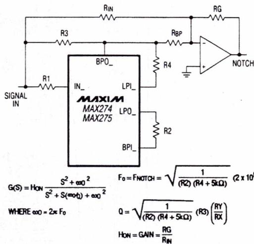
$$G(S) = H_{0N} \frac{S^2 + \omega_0^2}{S^2 + S(\omega_0 Q) + \omega_0^2}$$
