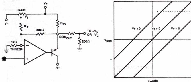
\*UPPER AND LOWER LIMITS CAN BE ESTABLISHED BY VALUES OF  $R_{PV}$  AND  $R_{LL}$ , RESPECTIVELY
